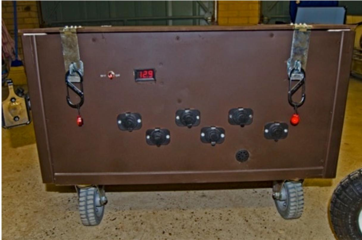
Back: GFCI outlet, inverter's power switch, air vent (for inverter) and 7-port USB hub
